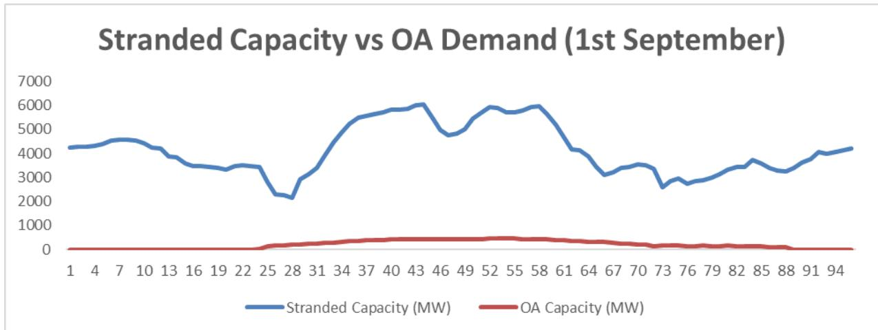
19. As observed, the pronounced bulge during solar hours reflects surplus RE injection into the grid, resulting in conventional capacity remaining idle or stranded across most months. Accordingly, it is not the migration of consumers to Open Access that leaves capacity unutilised; rather, it is the inherent intermittency of RE—surplus during solar hours and negligible generation during non-solar hours—that leads to stranding of long-term capacity.
